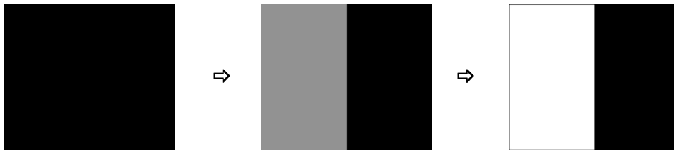
Fig. 9: Phase patterns used to determine the phase modulation.
